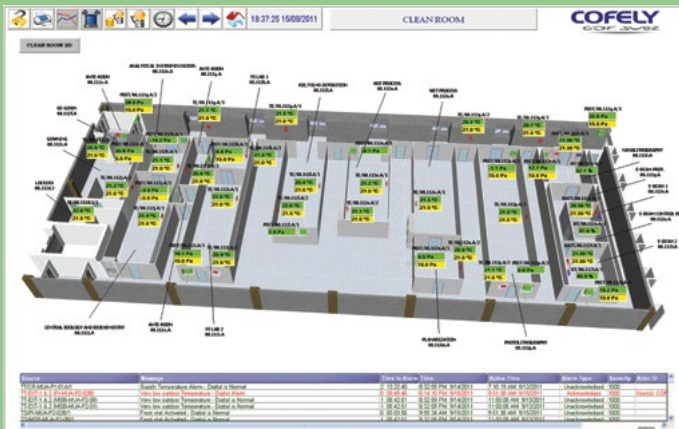
Clean Room Floor Monitoring/Control
