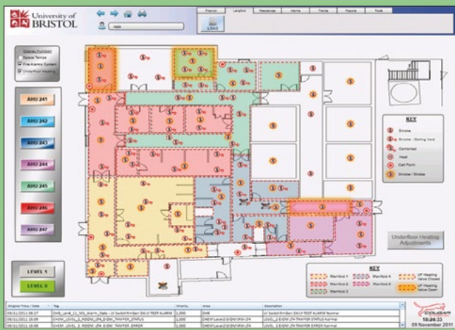
An AHU Zone Monitoring Display
