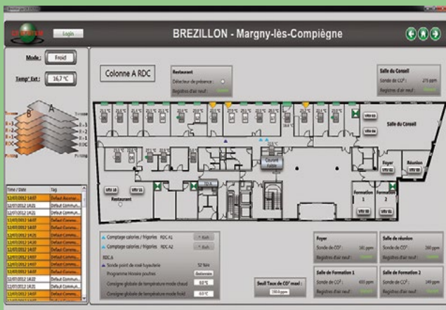
Building Temperature and CO2 Monitoring
