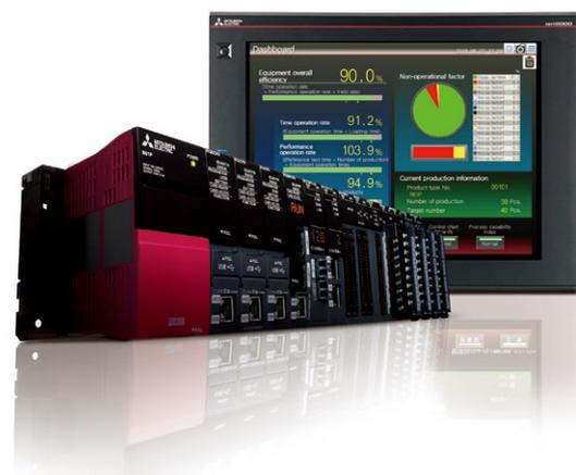
The e-F@ctory starter package is a package of sample projects for analyzing equipment information collected in the programmable controller and displaying analyzed results on the GOT (HMI). Designing complex analysis algorithms and graphs is unnecessary, realizing the equipment operation monitoring system at a lower cost.
