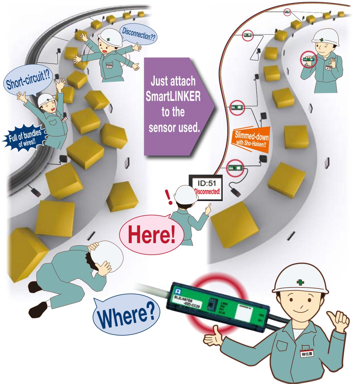
Intelligent Sho-Haisen that can detect sensor disconnection and short-circuit in real time
