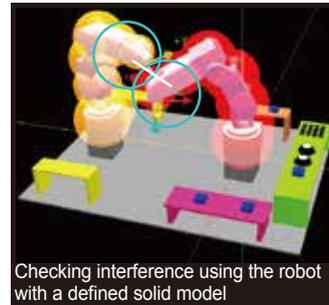
Checking interference using the robot with a defined solid model
