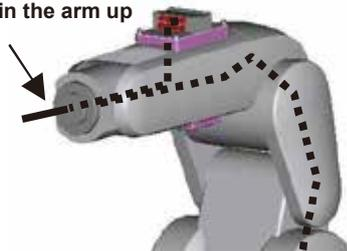
Note: Specify a model with Internal wiring (a model ending in '-SHxx').
