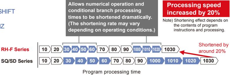
Robot programs can be executed 1.2 times faster than before if compiled in advance and processed using an intermediate language. Takt times can be shortened by up to 3 times as much for longer lines. (Compared to previous models)
