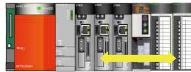
Direct control between CPUs and I/O units
