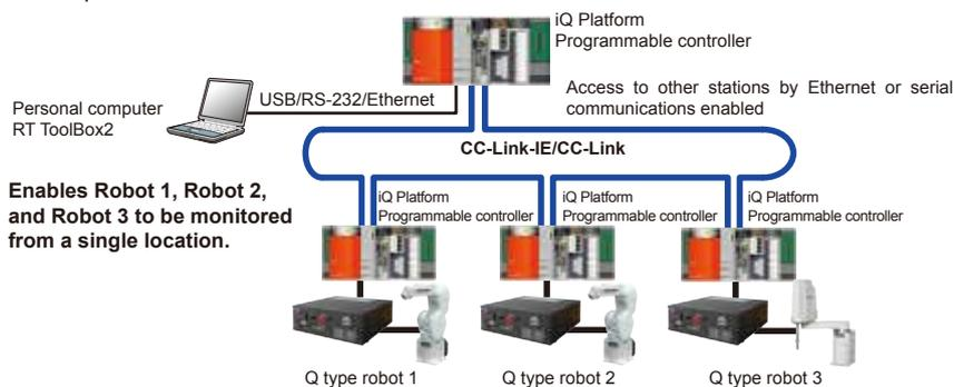
**Enables Robot 1, Robot 2, and Robot 3 to be monitored from a single location.**
