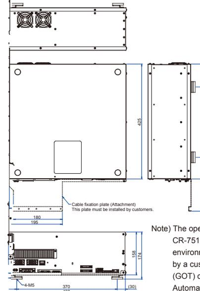
Note) The operating panel is not attached to the CR-751. Set up the robot operating environment to accommodate operation by a customer graphical optical terminal (GOT) or operating panel. Automatic and other operation modes can be enabled from the teaching pendant.
