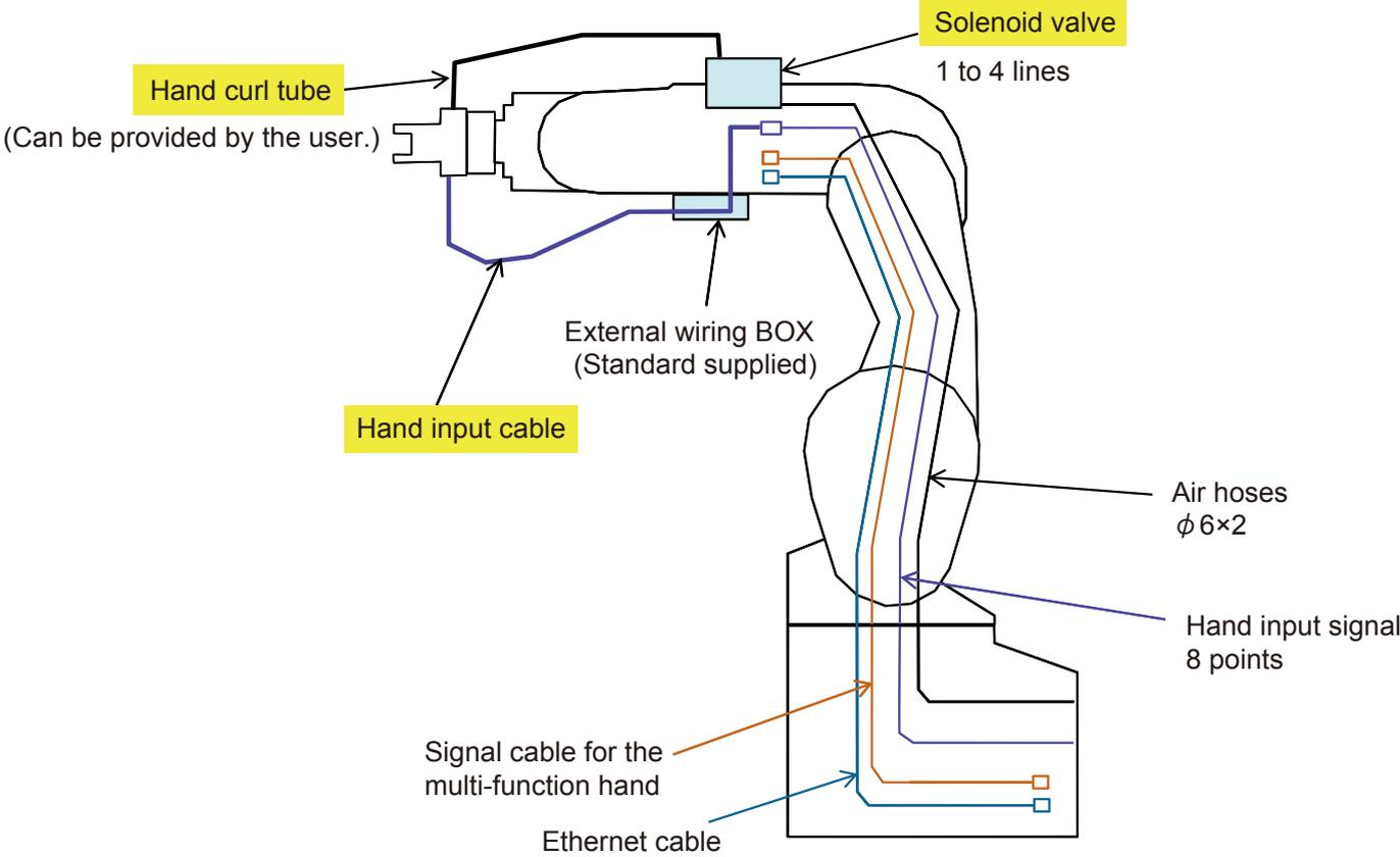
RV series Tooling (air-hand) : Internal wiring
