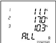
1<sup>st</sup> line: Side 1 distortion ratio (content rate)
