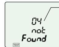
When incorrect wiring pattern cannot be detected
