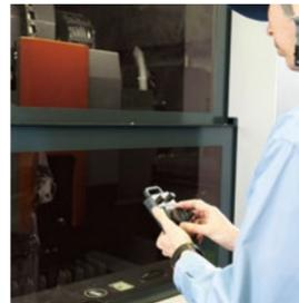
Adjusts the processing condition by a dial while looking at the processing.
