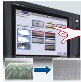
High quality processing regardless of proficiency is possible by selecting the similar picture to processing status.
