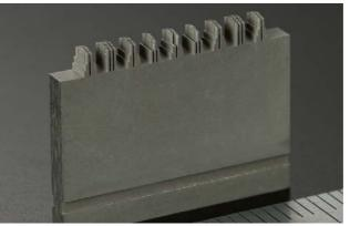
Wire electrode : ø0.05(.002")/SF Workpiece : Steel(PD613), Length 20mm(.79") width 2mm(.08")
