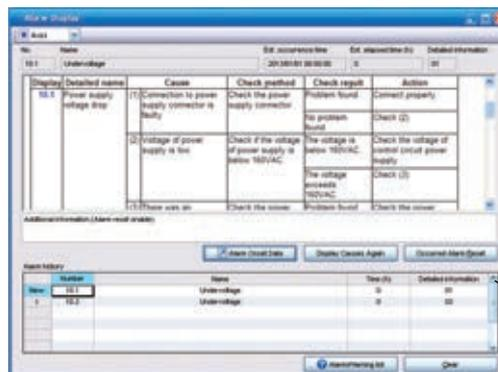
The alarm No. shows whether the undervoltage alarm was caused by instantaneous power failure or by lowered bus voltage in the servo amplifier.
