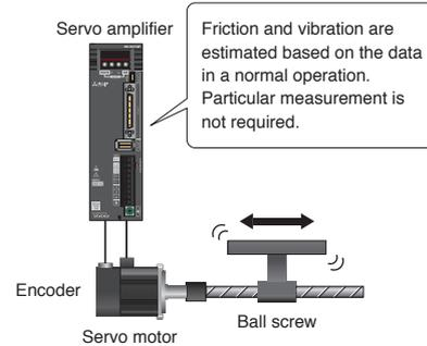
Friction and vibration are estimated based on the data in a normal operation. Particular measurement is not required.
