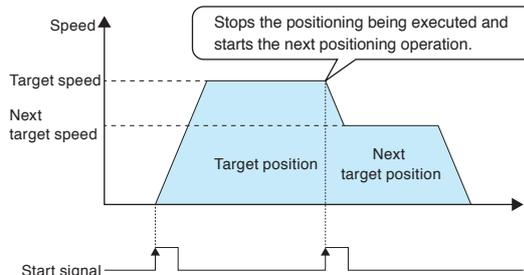
Equipped with positioning function
