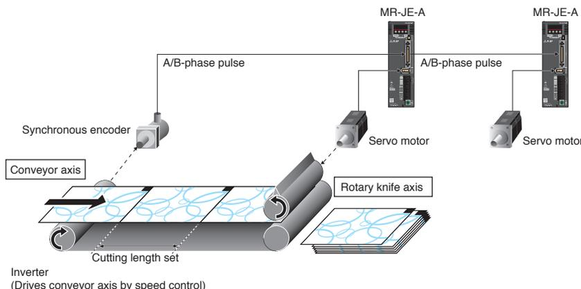
Compensating a position gap by sensor input
