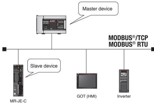
\* MODBUS® RTU is supported by servo amplifiers with software version A4 or later.
