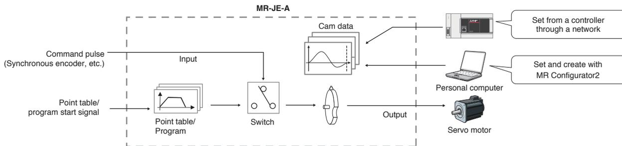
Synchronous simple operation by encoder signal input
