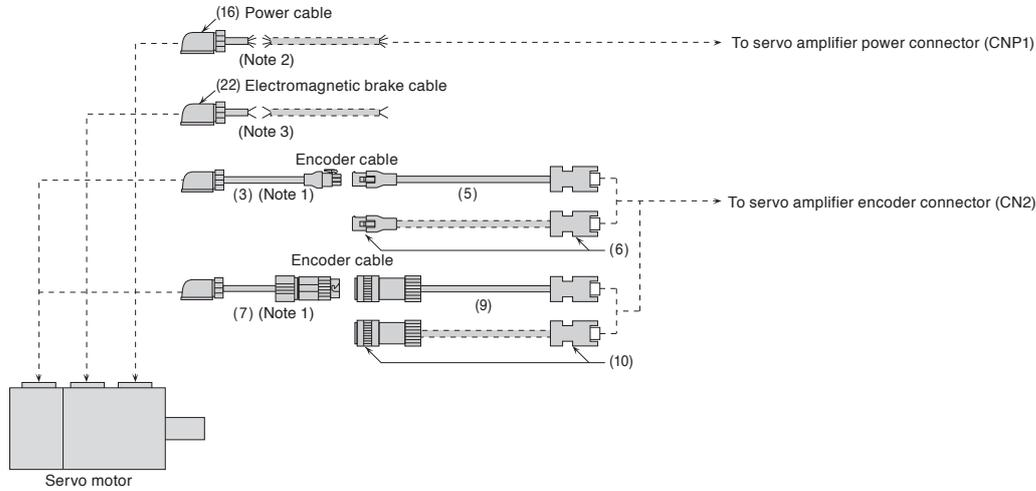
● For leading the cables out in opposite direction of load side (Note 4)
