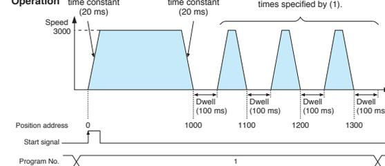
Automatic calculation of travel distance by setting the number of stations in parameter
