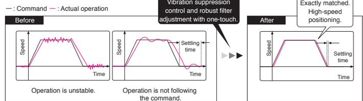
Suppressing two types of low frequency vibrations at once
