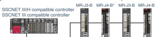
\* When the SSCNET III compatible products are in the system, the communication speed is 50 Mbps, and the function and the performance are equivalent to those of MR-J3.
