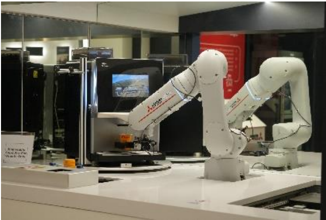
Image 5: Coffee serving using collaborative robot, MELFA Assista
