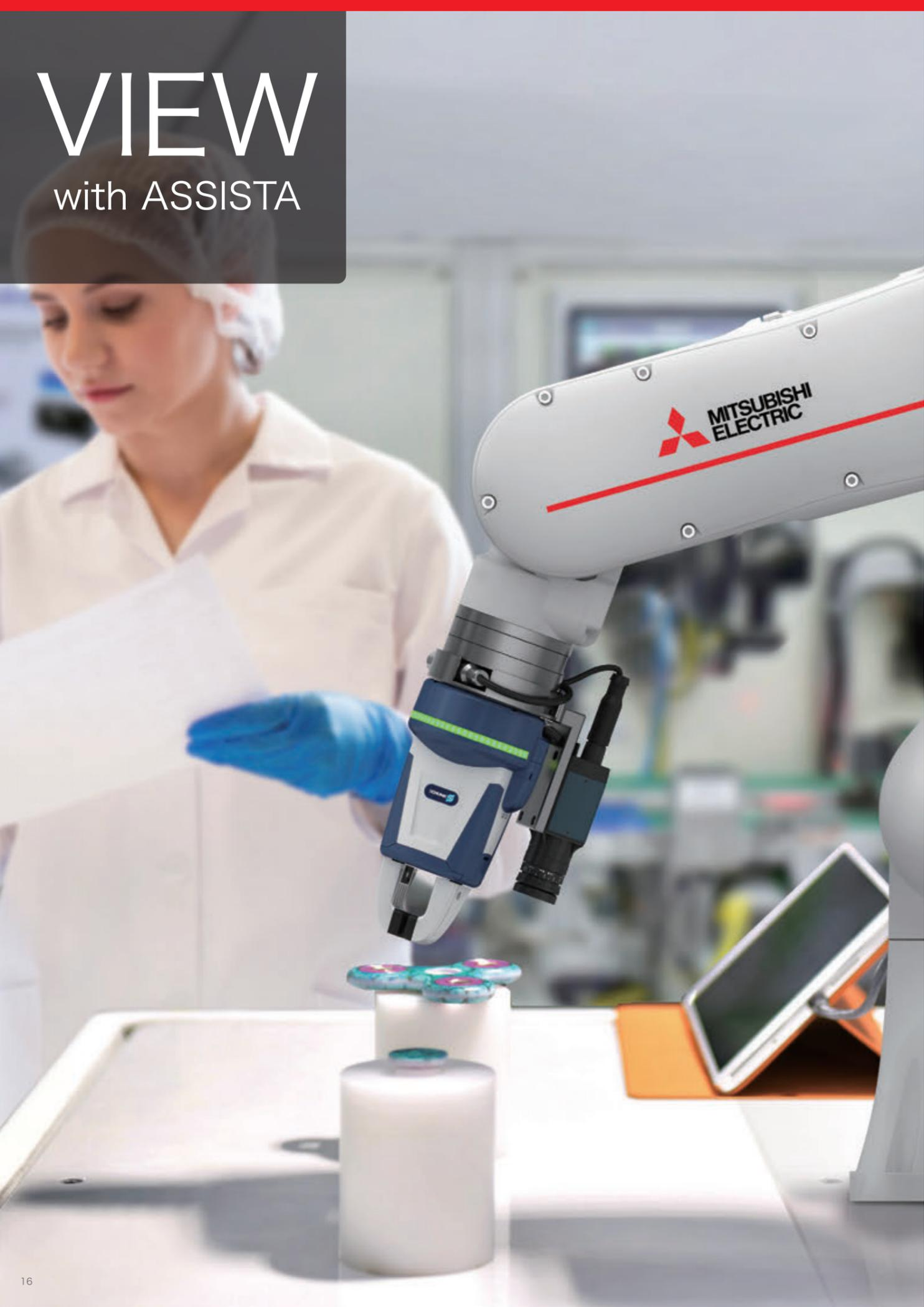
ASSISTA and the camera capture the target using the “RT VisualBox” auto-focus function.
