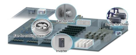
One example to increase energy efficiency is the use of inverters for motors that drive pumps and fans in the air conditioning systems
