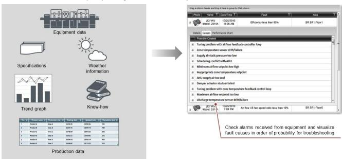
SCADA systems can be used to list-up potential fault causes in order of probability to make troubleshooting tasks easier - this example is from a GENESIS64 solution.
