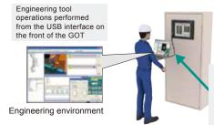
The personal computer and the GOT are connected with a USB cable or RS232 cable
