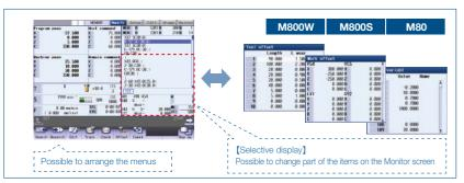
Standard screens can be customized using the selective display and rearranging menus. Screens matching operators' preferences and needs enable even greater ease of use.
