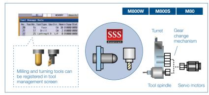
High-speed high-accuracy control and SSS control are available for milling using lathe system. A servo motor driven by a servo drive unit can be controlled as a tool spindle.
