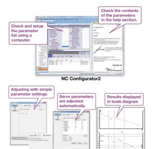
Servo parameters can be adjusted automatically by measuring and analyzing the machine's characteristics. Measurement and analysis can be done by running a servo motor using the machining program for adjustment, or using the vibration signal. This function can sample various types of data.
