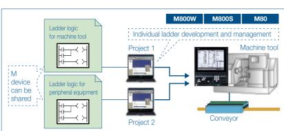
Multi-project PLC enables control of ladder logic for peripheral equipment separately from that for machine tools. This leads to efficient development and management of ladder logics for peripheral equipment.
