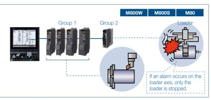
During an alarm, operation of individual machine groups can be stopped. Machining is not interrupted when an alarm occurs on peripheral equipment (e.g., loader).
