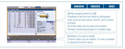
Tool-related information is collected and centrally managed on the Tool Management Screen. A wide range of setting items such as tool name and tool ID are readily available. It is also possible to add custom data.
