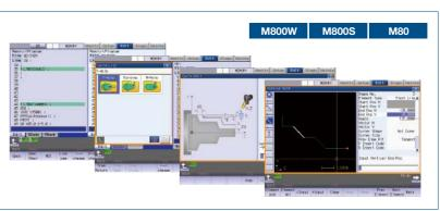
Conversational programming, tool measurement, work coordinate system shift and other features have been improved, making the lathe system significantly easier to use.
