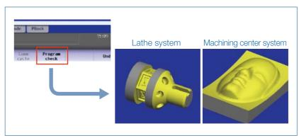
A click of the menu button navigates you to 3D graphic check of the currently edited program. For lathe system, the 3D check supports for both milling and turning.
