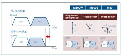
Rapid traverse block overlap function makes it possible to reduce non-cutting time. The overlap varies according to the path to keep the tolerance constant.
