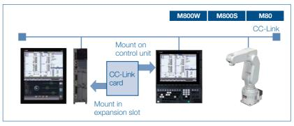
Compatible with CC-Link (master/slave), PROFIBUS-DP (master) Possible to connect to peripheral equipment and devices conforming to a range of field networks.
