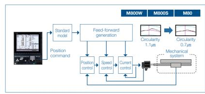
"OMR-FF control" makes servo control smoother and more accurate, enabling optimal position loop gain adjustment suited to each axis.
