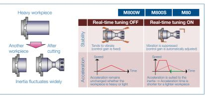
Real-time tuning helps maintain the stability of large lathes. This function detects vibration caused by significant fluctuation of work inertia and automatically adjusts the control gain.
